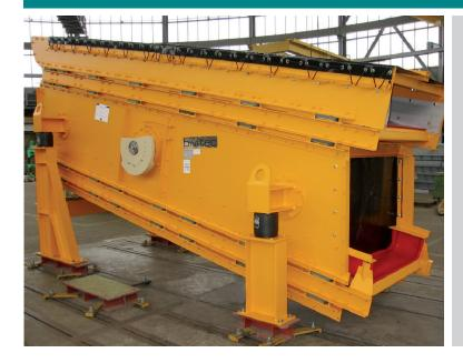
Using special screening machines in the Dorste plant of Südharzer Gipswerke GmbH to implement a finer cut point, thus increasing product output.
